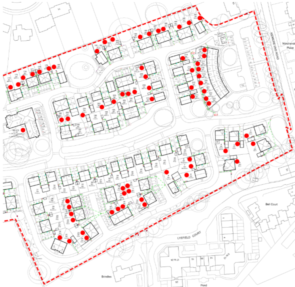
Plan showing location of dwellings to be served by air source heat pumps within the development (red circles)
