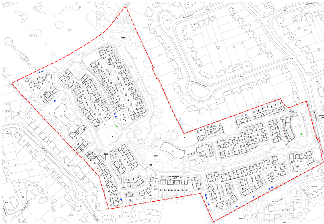
Plan showing layout of 13 x Visitor (blue dots) & 2 x Car Club (green dots) Parking Spaces
