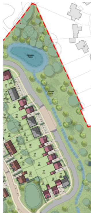
Proposed location of attenuation swale, in northeast corner of site, including crossing points
